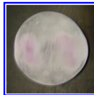
FIGURE 9: Traditional etch of SPnfe6. A hemisphere mounted with its secondary prism plane normal to the ice finger was grown in the presence of 0.1 mg/mL tetramethylrhodamine-labeled SPnfe6. Two distinct protein patches, oriented in the same manner as observed with GFP-SPnfe6 (Figure 3), were revealed on the surface of the crystal after the hemisphere was allowed to sublime at -20^{\circ} C for ca. 24 h. Each patch has a faint pink color resulting from the inherent fluorescence of the tetramethylrhodamine label viewed under normal light.
